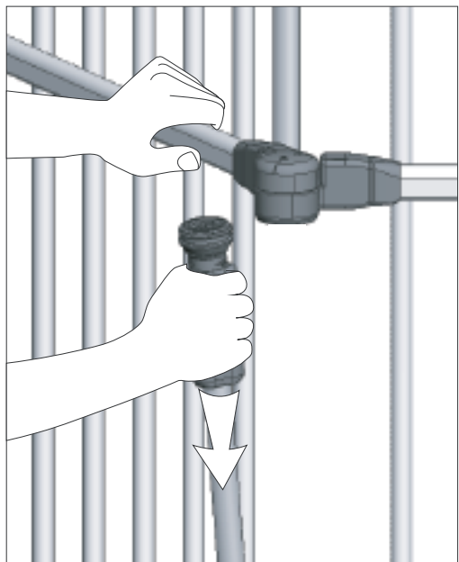
Step 3: Remove the vertical bars in both panels you wish to connect. Turn clockwise to loosen and pull down to remove.
