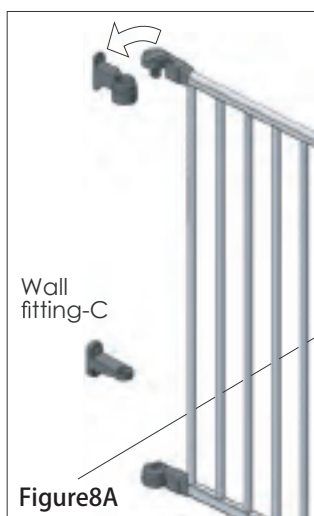
Wall fittings - A side
