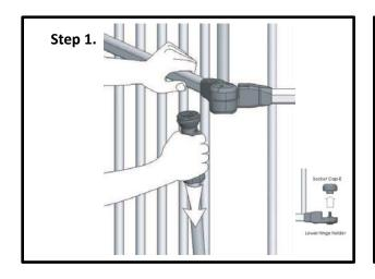
Remove the vertical bar from one end on the extension and the panel you wish to connect. Turn clockwise to loosen and pull down to remove. **Note:** If applicable, remove the Socket Cap E.
