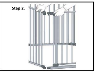
To connect the panels together, vertically lift one panel allowing the upper and lower hinge housings to slip into place in the mating panel.
