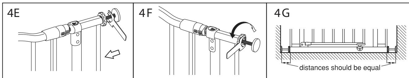
**Note:** When tightening, the distance between the 4 tension bolts should be equal, as shown in figure 4G.
