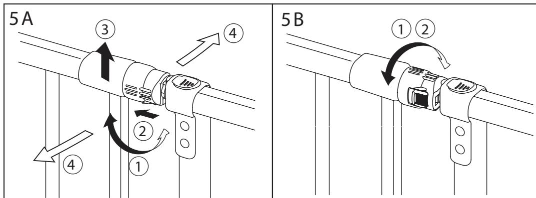
**Note:** Verify proper gate installation by partially opening and releasing it several times. The door will swing closed and double-latch automatically. Regularly check tension knobs and rubber pads to make sure the gate is securely in place.
