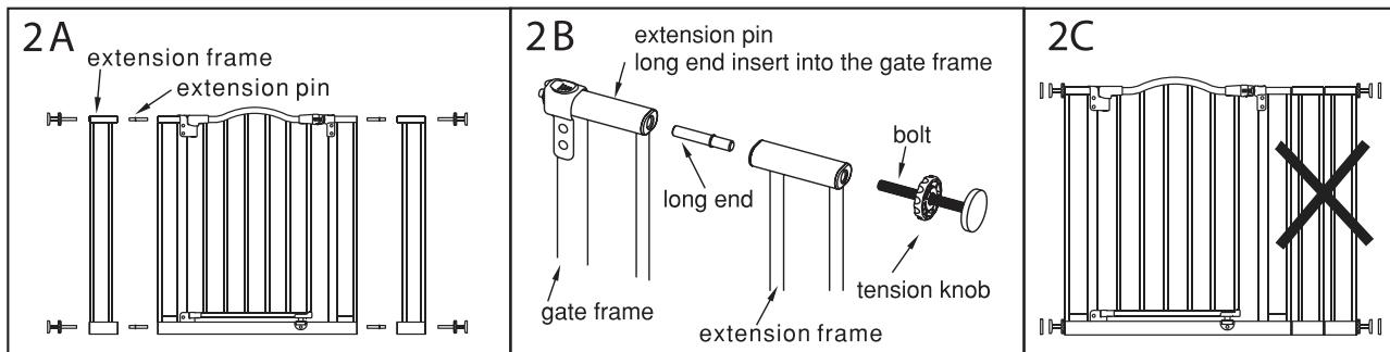
**IMPORTANT:** Do not install two extensions on the same side of the gate, as shown in figure 2C.
